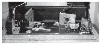
Figure 3. Photograph of the spectrograph. The chassis is a  $60 \times 90$  cm black granite slab drilled for threaded inserts at strategic locations. The mirrors are mounted on the left, the diffraction grating on the lower right, and the CCD is on the upper right.
